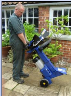
A variable height table allows logs of up to 1 metre in length to be split or 1.25 metres with the Eco85
