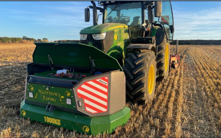
Standard Workbox with detachable 1000kg BellyWeight
