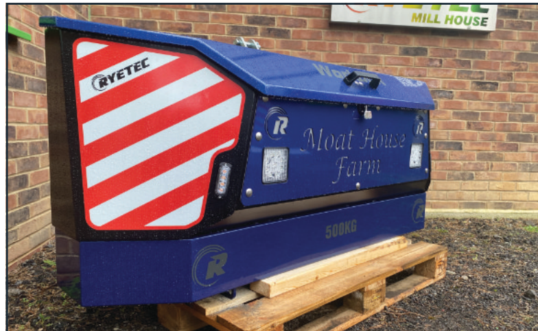
Detachable belly weights for when extra weight is required
