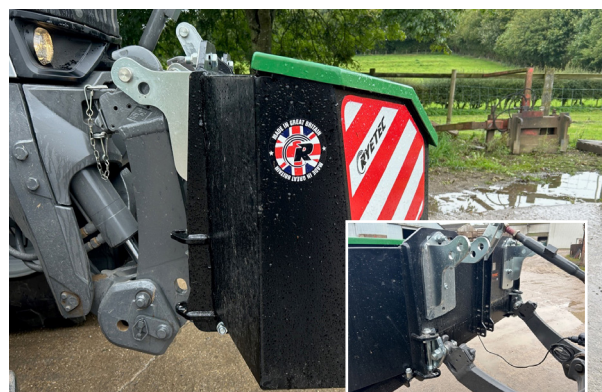
Unique interchangeable linkage mount as standard
