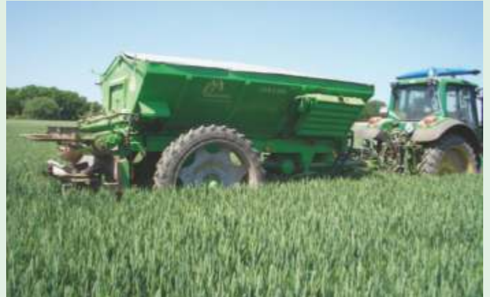
Crop top dressing with electronically controlled hydraulically powered Güstrower spreader combined with „Yara - N - Sensor“.
