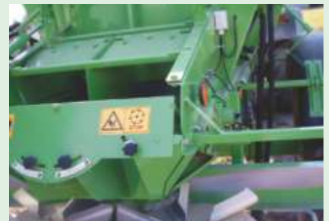
Remote hydraulic door to stop spillage of high volume free running material during road transport.
