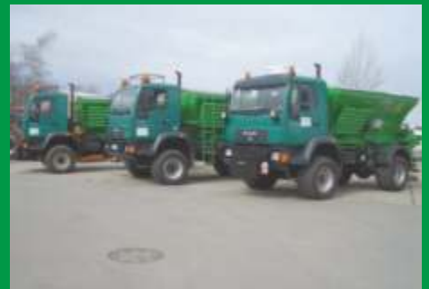
At 14 to - MAN mounted spreaders (client is a contractor).
