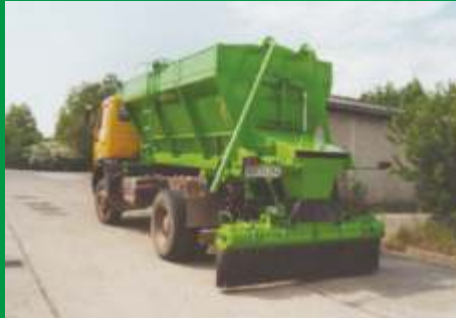
Mounted spreader for soil stabilisation.
