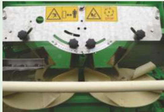
Stainless steel guide plates control exactly where fertiliser drops on the spreading vanes.
