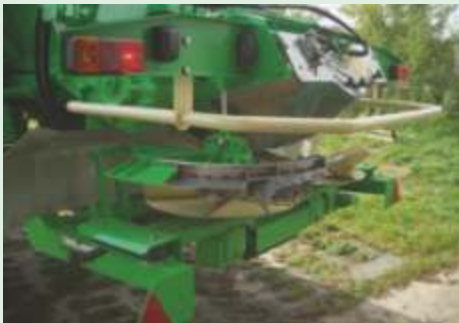
Hydraulically operated border control.
