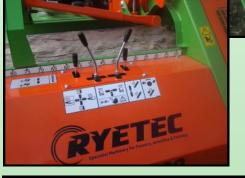
Central operator station with convenient two handed joystick controls
