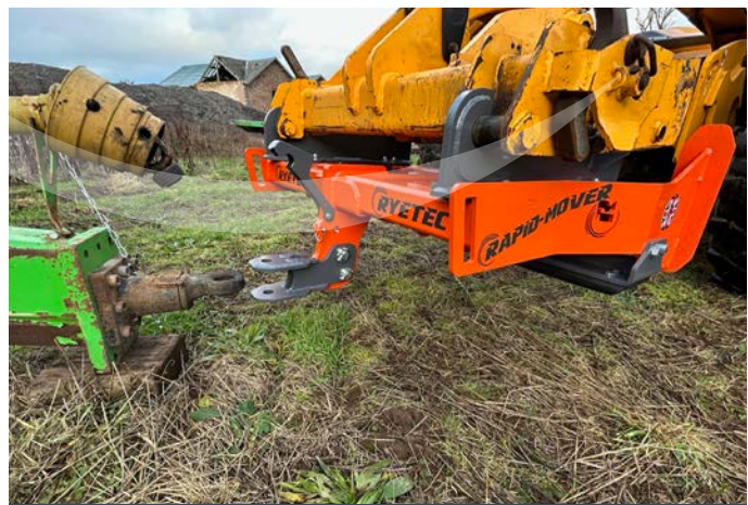
Fold out clevis hitch to move trailed implements with ease
